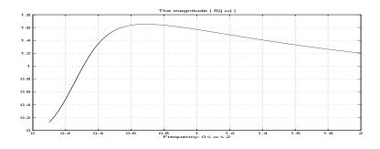
Figure 1: PI control of integrating plus time delay process,  $h_p(s) = k \frac{e^{-\tau s}}{s}$ with gain k = 1 and time delay  $\tau = 1$ . PI-controller  $h_c(s) = K_p \frac{1+T_i s}{T_i s}$  with settings  $K_p = 0.4004$  and  $T_i = 4.9953$ . The figure illustrates the magnitude of the frequency response of the sensitivity transfer function as a function of frequency. The sensitivity index  $M_s$ , i.e., the maximum peak and for this system given by  $M_s \approx 1.6515$ .
