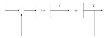
Figure 1: Standard feedback control system.
