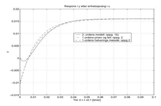
Figure 1: Unit step-response for the model in (9) and the approximate 1st order models in task 2 after unit step in u. The figure is generated by the MATLAB script file **demo\_reac\_pid.m**. Se the enclosed MATLAB file.
