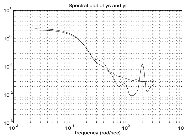
Figure 5.10: The estimated frequency function of the actual stochastic part of the power model, i.e. y^s = y - y^d , and \hat{y}^d .
